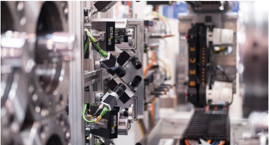
Inspection system specially designed for the quality assurance of in-mold labels
