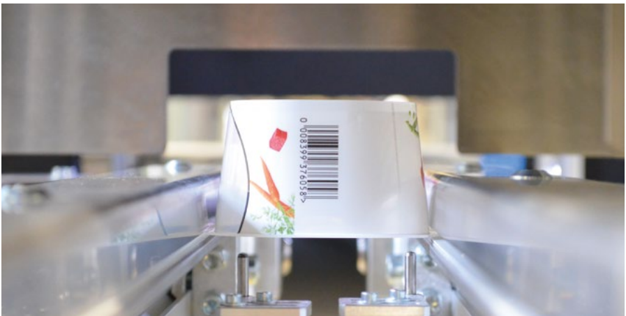
Making invisible defects visible: Non-destructive inspection of EVOH barrier layers
